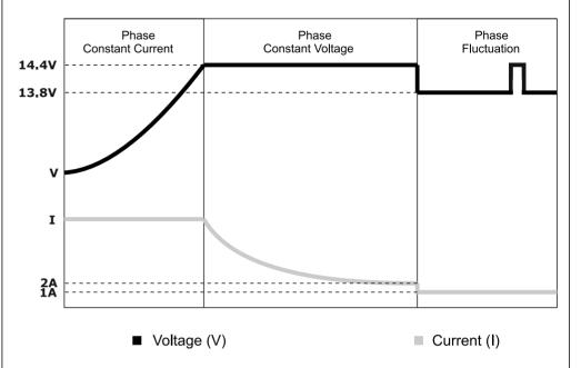
**Constant Current Phase** - The current is constant keeped while the voltage up until the point when happens the electrolyte's decomposition; At the final phase, the battery has around 75~80% of his nominal capacity.
